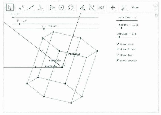
An examination of the construction protocol shows that the appearance of 3 D graphics is obtained by working with a list of points, using matrix multiplications for the rotations, and projections of the points into a plane.
