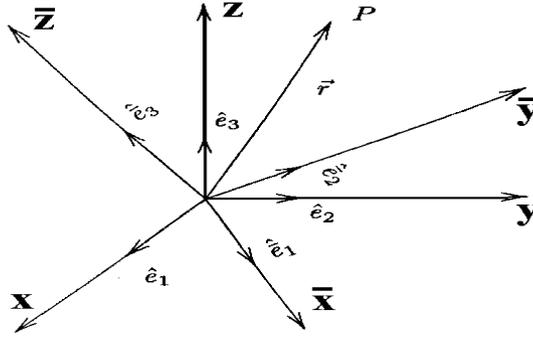
Figure 1.3-15. Rotation of axes
