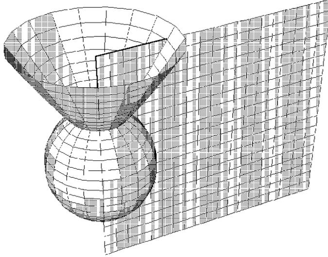
Figure 1.3-9. Prolate spheroidal coordinates
