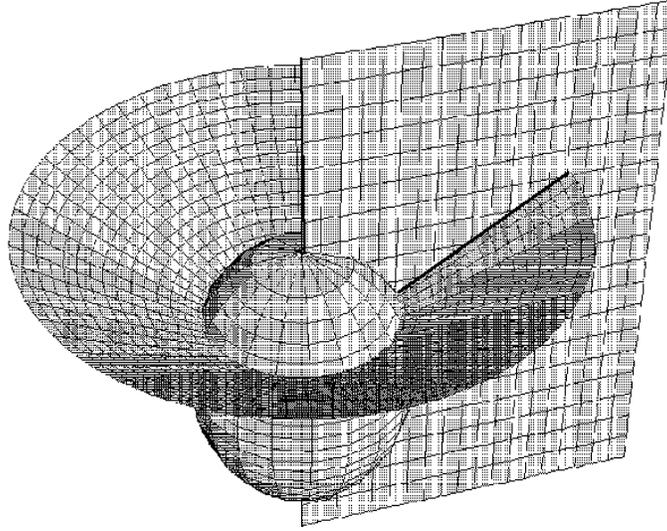
Figure 1.3-6. Elliptic coordinates  $\phi = \pi/4$ .
