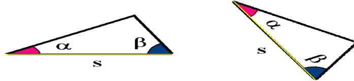
Figure 2-14. Angle-Side-Angle required for two triangles to be congruent
