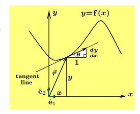
Note that at the point (x, f(x)) on the curve one can draw the derivative vector and show that it lies along the tangent line to the curve at the point (x, f(x)). This shows that the derivative  $\frac{d\vec{r}}{dx}$  is a tangent vector to the curve y = f(x).
