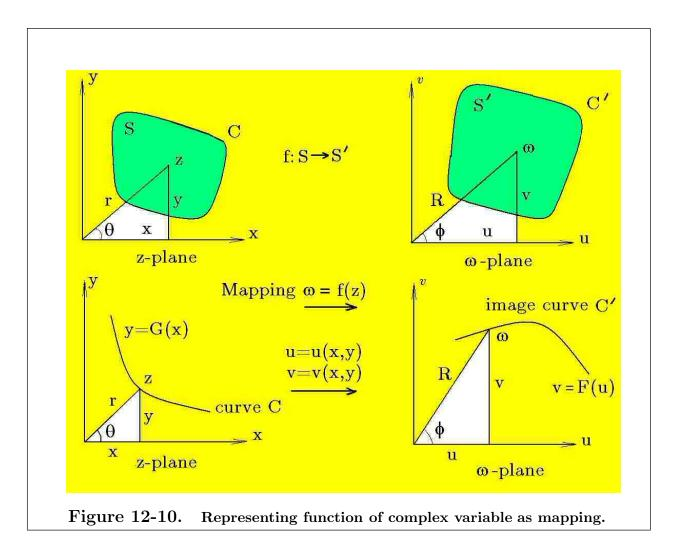
Polar coordinates  $(r,\theta)$  in the z-plane correspond to polar coordinates  $(R,\phi)$  in the  $\omega$ -plane, where  $x=r\cos\theta,\ y=r\sin\theta$  in the z-plane and  $u=R\cos\phi,\ v=R\sin\phi$  in the  $\omega$ -plane. A curve y=G(x) in the z-plane has the image curve with parametric form
