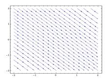
Streamlines  $\sin \alpha x + \cos \alpha y = c$  and velocity field is derivable from potential function  $\phi = V_0 \cos \alpha x - V_0 \sin \alpha y$
