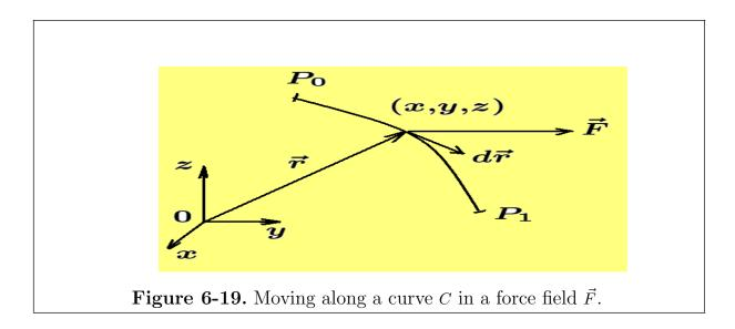
Examine the particle at a general point (x, y, z) on the given curve C. Construct the position vector  $\vec{r}$ , the force vector  $\vec{F}$ , and the tangent vector  $d\vec{r}$  acting at this general point on the curve. The line integral
