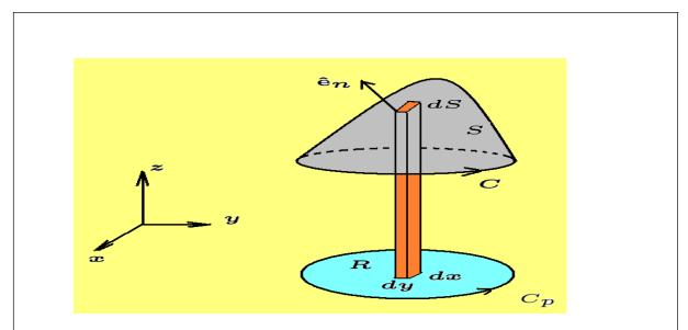
**Figure 8-13.** Surface S bounded by a simple closed curve C on the surface.
