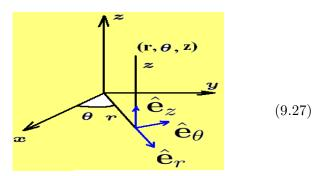
obtained from equations (7.107), the position vector of a moving particle can be expressed in cylindrical coordinates as
