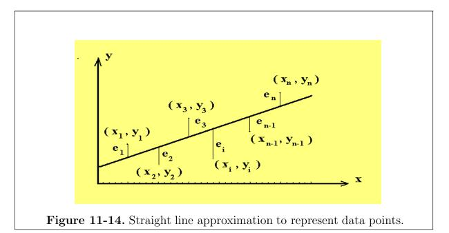
One way to define the "best" straight line  $y = \beta_0 + \beta_1 x$  is to select the constants  $\beta_0$  and  $\beta_1$  which minimize the sum of squares of the errors associated with the data set. That is, if
