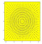
▶ 9-9. Integrate the equations  $\frac{\partial \phi}{\partial x} = \frac{-ky}{x^2 + y^2}$  and  $\frac{\partial \phi}{\partial y} = \frac{kx}{x^2 + y^2}$  to obtain
