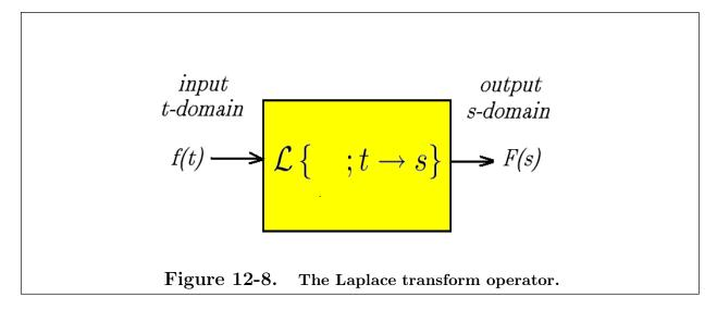
In the defining equation (12.175) the parameter s is selected such that the integral exists and many times it is expressed as a complex variable  $s = \sigma + i\omega$  where  $\sigma$  and  $\omega$  are real and i is an imaginary component satisfying  $i^2 = -1$ . The Laplace transform can be studied with or without employing knowledge of complex variables.
