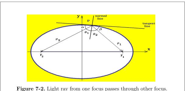
The position vector of a general point on the ellipse can be represented in the parametric form
