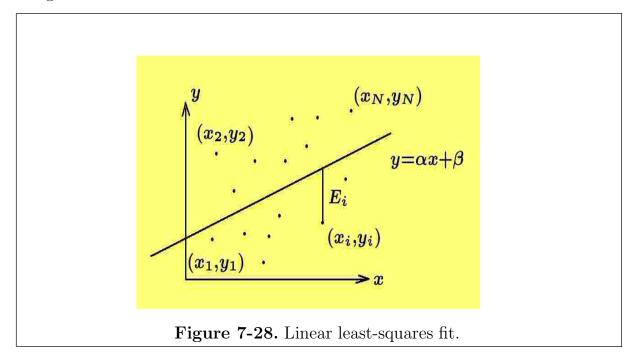
Each data point  $(x_i, y_i)$  has associated with it an error  $E_i$  which is defined as the difference between the y value of the line and the y value of the data point. For example, the error associated with the data point  $(x_i, y_i)$  can be written
