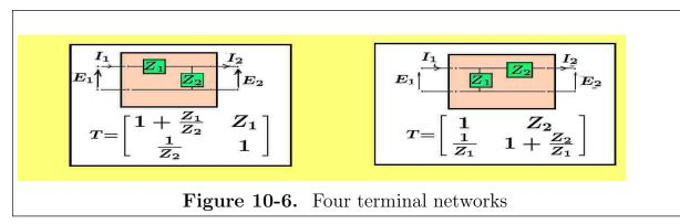
In figure 10-6 the quantities  $I_1$ ,  $E_1$  and  $I_2$ ,  $E_2$  are the input and output current and voltages. The column vectors  $S_1 = \text{col}[E_1, I_1]$  and  $S_2 = \text{col}[E_2, I_2]$  are called the input state vector and output state vector of the network. The networks are assumed to be linear so that the general relation between the input and output states can be expressed as the matrix equation
