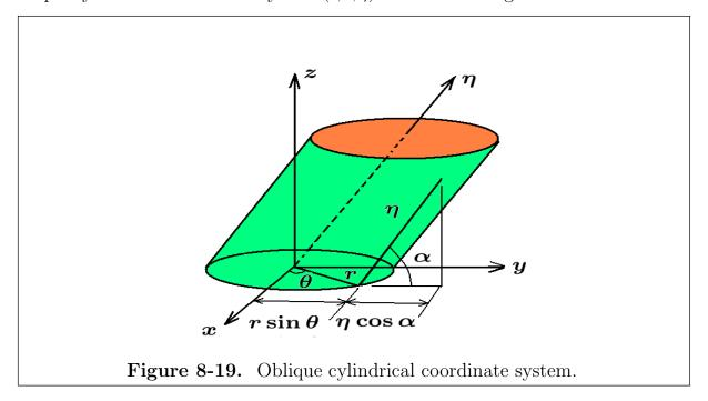
The transformation equations (8.68) are obtained from the geometry in figure 8-19. These equations are
