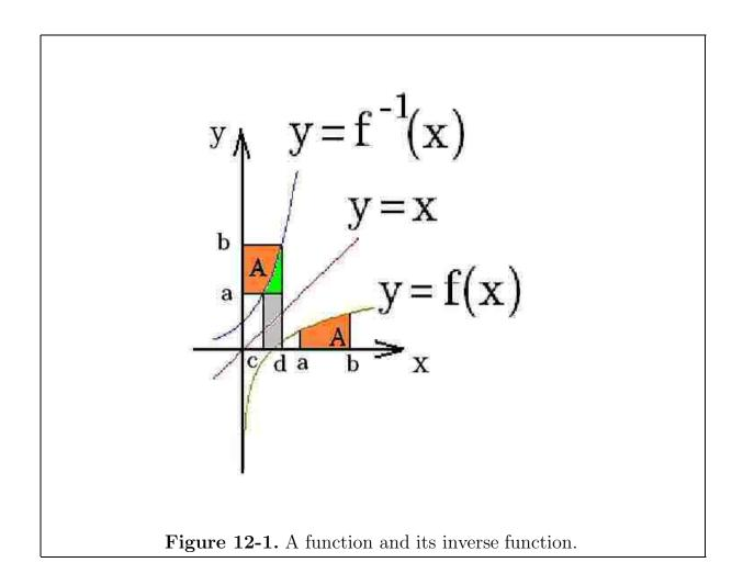
We know that the functions f(x) and  $f^{-1}(x)$  are symmetric about the line y = x as illustrated in the figure 12-1. Examine the figure 12-1 and note that one can express the area  $A = \int_a^b f(x) dx$  as
