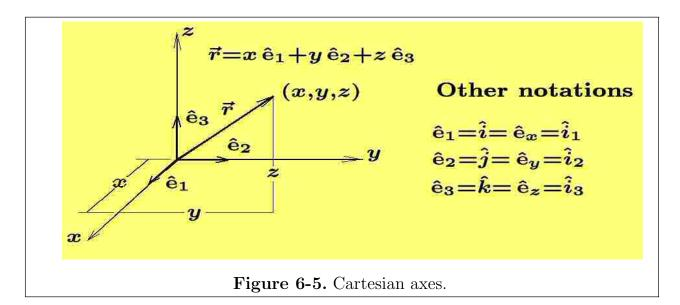
The figure 6-5 illustrates unit base vectors  $\hat{\mathbf{e}}_1$ ,  $\hat{\mathbf{e}}_2$ ,  $\hat{\mathbf{e}}_3$  in the directions of the positive x, y, z-coordinate axes in a rectangular three dimensional cartesian coordinate system. These unit base vectors in the direction of the x, y, z axes have historically
