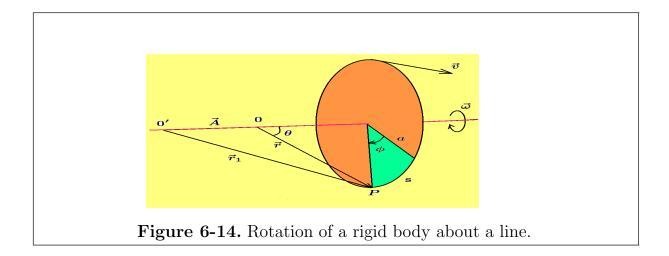
The geometry in figure 6-14, is investigated and indicates that  $a = |\vec{r}| \sin \theta$ , and hence the magnitude of the velocity can be represented as
