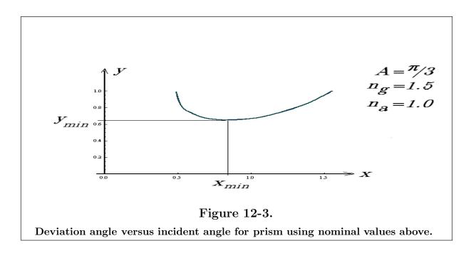
An alternative approach of finding the value of x which produces a minimum value is as follows. Observe that when  $y = y_{min}$ , then  $\frac{dy}{dx} = 0$ . Assume that y has the value  $y = y_{min}$  and differentiate the equations (12.12) and (12.13) with respect to x and show
