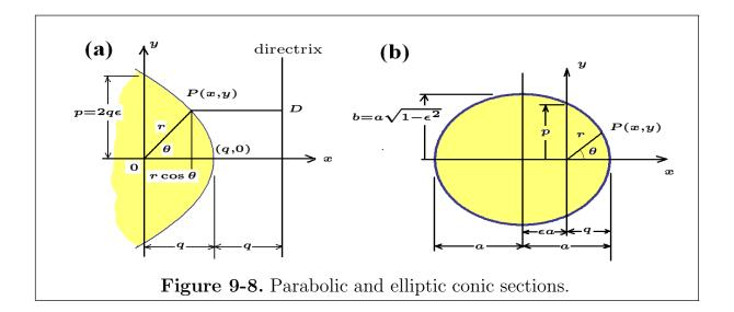
With reference to figure 9-8, a conic section is defined in terms of the ratio  $\frac{\overline{OP}}{\overline{PD}} = \epsilon$ , where  $\overline{OP} = r$ , and  $\overline{PD} = 2q - r\cos\theta$ . From this ratio, solve for the radius r and obtain the representation
