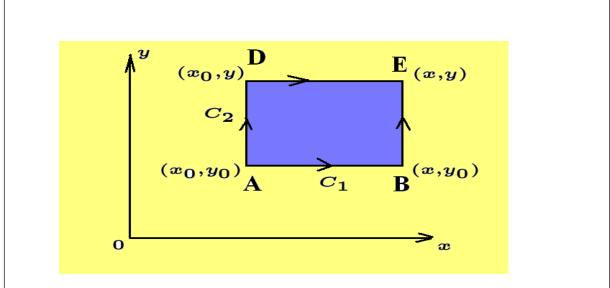
Figure 8-10. Path of integration for solution to exact differential equation.
