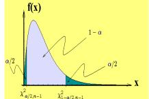
Secondly, one must calculate the variance squared  $s^2$  using equation (11.82), then construct the confidence interval for the variance of a normal distribution given by
