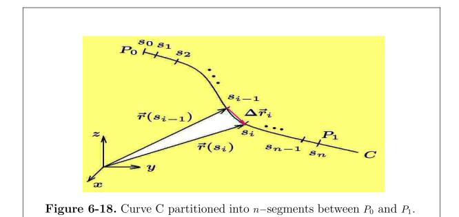
The above formulas result indirectly from the following limiting process. On that part of the curve between the given points  $P_0(x_0, y_0, z_0)$  and  $P_1(x_1, y_1, z_1)$ , the arc length along the curve is divided into n segments by a set of numbers
