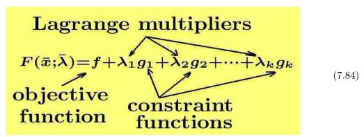
which contains the objective function f, summed with each of the constraint functions  $g_i$ , multiplied by a Lagrange multiplier  $\lambda_i$ , for the index i having the values i = 1, ..., k. Here the function F and consequently the function f has stationary values at those points where the following equations are satisfied
