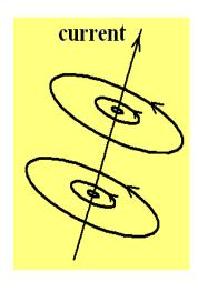
A moving charge produces a current and a moving current produces a magnetic field. Consider a current moving along a wire considered as a line. The magnetic field created is described by circles around the wire. The strength of the magnetic field falls off as the perpendicular distance from the line increases. One can use the right-hand rule of letting the thumb point in the direction of the current flow, then the fingers of the right-hand point in the direction of the magnetic field lines.
