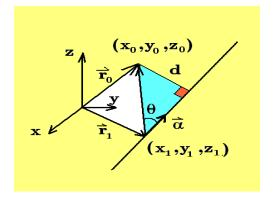
Define the unit vector  $\hat{\mathbf{e}}_{\alpha} = \frac{1}{|\vec{\alpha}|} \vec{\alpha}$  and construct the line from  $(x_0, y_0, z_0)$  which is perpendicular to the given line and label this distance d. Our problem is to find the distance d. From the geometry of the right triangle with sides  $\vec{r}_0 - \vec{r}_1$  and d one can write  $\sin \theta = \frac{d}{|\vec{r}_0 - \vec{r}_1|}$ . Use the fact that by definition of a cross product one can write
