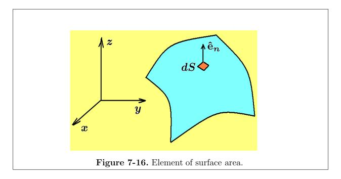
In the representation of various vector integrals, it is convenient to define vector elements of surface area  $d\vec{S}$  whose magnitude is dS and whose direction is the same as the unit outward normal  $\hat{\mathbf{e}}_n$  to the surface. Define this vector element of surface area as  $d\vec{S} = \hat{\mathbf{e}}_n dS$  which can be considered as the limit associated with the area  $\vec{\Delta}S = \hat{\mathbf{e}}_n \Delta S$ .
