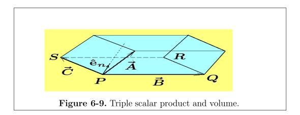
(c) The dot product  $\vec{A} \cdot \hat{\mathbf{e}}_n = \vec{A} \cdot \frac{\vec{B} \times \vec{C}}{|\vec{B} \times \vec{C}|} = h$  represents the projection of  $\vec{A}$  on  $\hat{\mathbf{e}}_n$  and produces the height of the parallelepiped. These results demonstrate that
