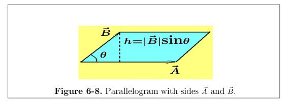
The area of the parallelogram having the vectors  $\vec{A}$  and  $\vec{B}$  for its sides is given by
