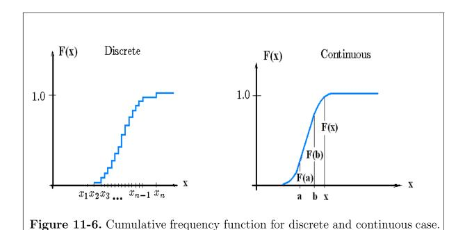
In both the discrete and continuous cases the cumulative frequency function represents the probability
