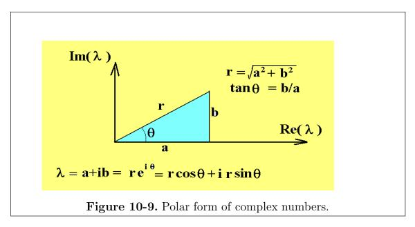
In this figure r is called the modulus or length of the complex number  $\lambda$  and  $\theta$  is called an argument of the complex number  $\lambda$ . Values of  $2\pi$  can be added to obtain other arguments of  $\lambda$ . A value of  $\theta$  satisfying  $-\pi < \theta \le \pi$  is called the principal value of the argument of  $\lambda$ . The complex root  $\lambda_1$  has a modulus and argument of
