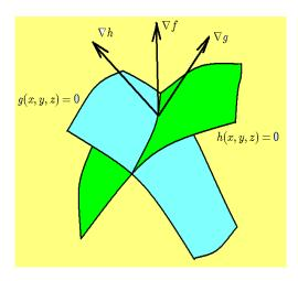
The method of Lagrange multipliers can be applied in higher dimensions. For example, consider the problem of finding maximum and minimum values associated with a function f = f(x, y, z) subject to the constraint conditions g(x, y, z) = 0 and h(x, y, z) = 0. Here the equations g(x, y, z) = 0 and h(x, y, z) = 0 describe two surfaces that may or may not intersect. Assume the surfaces intersect to give a space curve.
