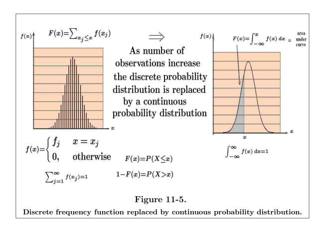
The function  $F(x) = \sum_{x_j \le x} f(x_j)$  is called the **cumulative frequency function** associated with the discrete sample. In the continuous case it is called the distribution function F(x) and calculated by the integral  $F(x) = \int_{-\infty}^{x} f(x) \, dx$  which represents the area from  $-\infty$  to x under the probability density function. These summation processes are illustrated in the figure 11-6.
