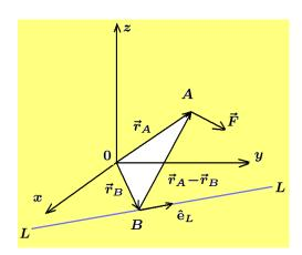
Assume one has a force  $\vec{F}$  acting through a given point A and  $\vec{r}_A$  is the position from the origin to the point A. The moment about the origin is given by  $\vec{M}_0 = \vec{r}_A \times \vec{F}$ . The moment of the given force  $\vec{F}$  about the lines representing the x, y and z axes are given by the projections of  $\vec{M}_0$  on each of these axes. One finds these moments
