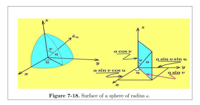
The position vector of a point on the surface of this sphere can be represented by the vector
