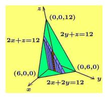
The figure on the left is a copy of the figure 7-20 with summations of the element dV illustrated. From this figure the limits of integration can be determined. The volume element is dV = dxdydz is placed at the general point (x, y, z) within the volume. This volume element can be visualized as a cube inside the volume. Summation of these cu-
