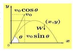
**Solution:** Let y = y(t) denote the vertical height at any time t and let x = x(t) denote the horizontal distance at any time t. Consider the cannon ball at a position (x, y) and examine the forces acting on it. In the y-direction the force due to the weight of the cannon ball is W = mg,  $(g = 32 \text{ ft/sec}^2)$ . The equation of motion in the y-direction is represented as
