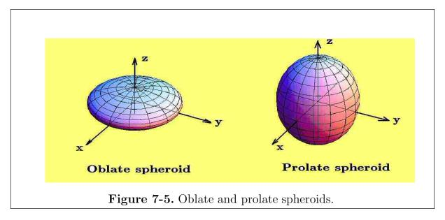
The ellipsoid can also be represented by the parametric equations
