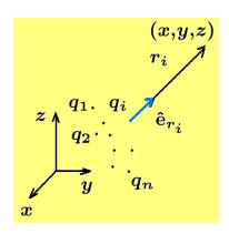
where  $\hat{\mathbf{e}}_{r_i}$ , for i = 1, ..., n, are unit vectors pointing from charge  $q_i$  to the point (x, y, z) of the test charge Q. The quantity
