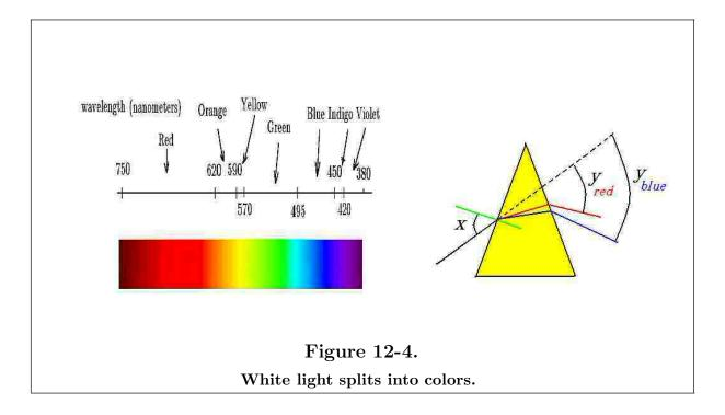
Recall that white light gets split into the colors Red, Orange, Yellow, Green, Blue, Indigo, Violet, remembered using the acronym (ROY G BIV). This is because the deviation angle for red light is less than the deviation angle for violet light. One can observe this by expressing the index of refraction in terms of the frequency  $(\nu)$  and wavelength  $(\lambda)$  of the light. The refraction index being given by
