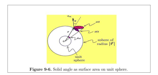
The solid angle subtended at the origin does not depend upon the size of the sphere about the origin and so one can write
