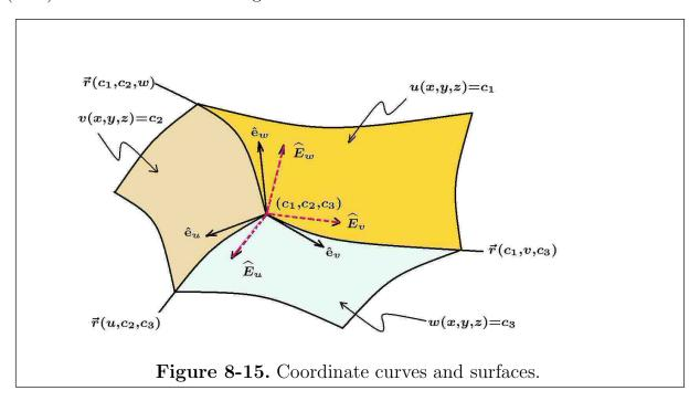
Consider the point  $u = c_1$ ,  $v = c_2$ ,  $w = c_3$  in the curvilinear coordinate system. This point can be viewed as being created from the intersection of the three surfaces
