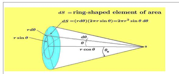
Figure 9-7. Area of spherical cap using ring-shaped element of area.
