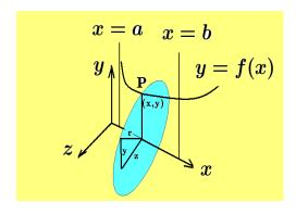
**Solution** A general point P on the given curve, when rotated about the x-axis produces the circle  $y^2 + z^2 = r^2$ , where r = f(x) is the radius of the circle. Eliminating the parameter r gives the equation of the surface of revolution as  $y^2 + z^2 = [f(x)]^2$
