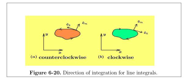
The direction of integration around a simple closed curve can be referenced with respect to the unit outward normal  $\hat{\mathbf{e}}_n$  and to the unit tangent vector  $\hat{\mathbf{e}}_t$  to the simple close curve as the direction of the unit tangent produces an oriented simple closed curve.
