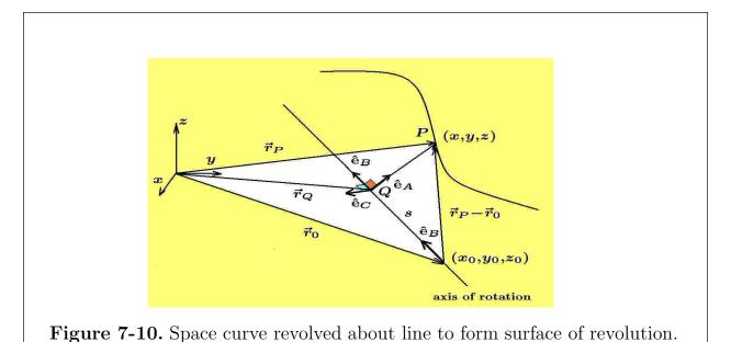
Consider a line perpendicular to the axis of rotation and passing through the point P. Denote by Q the point where this line intersects the axis of rotation. The distance s from the point  $(x_0, y_0, z_0)$  to the point Q is given by the projection of the vector  $\vec{r}_P - \vec{r}_0$  onto the unit vector  $\hat{\mathbf{e}}_B$ . This projection gives the distance
