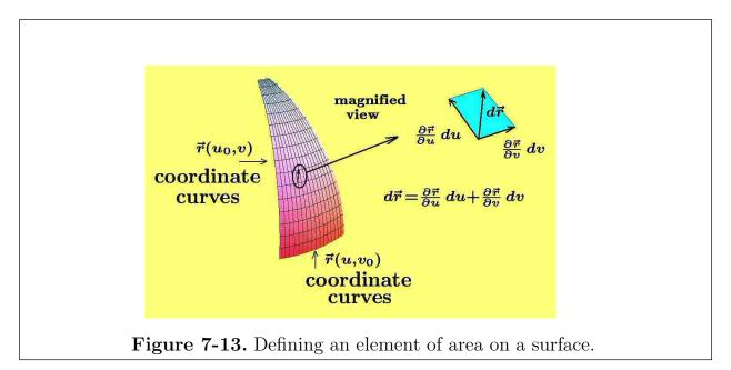
Define the element of surface area dS on a given surface as the area of the elemental parallelogram formed using the vector components of  $d\vec{r}$ . Recall that the magnitude
