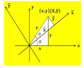
The above transformation equations between the  $(\bar{x}, \bar{y})$  axes which have been rotated through an angle  $\theta$  with respect to a fixed set of (x, y) axes can be represented by the matrix equation
