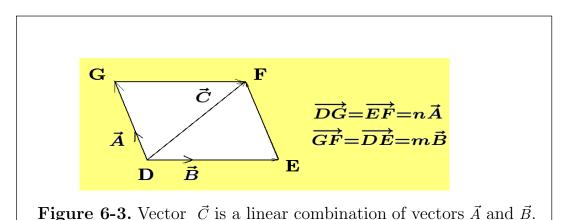
Since the vector side  $\overrightarrow{DE}$  is parallel to  $\overrightarrow{B}$  and the vector side  $\overrightarrow{EF}$  is parallel to  $\overrightarrow{A}$ , then there exists scalars m and n such that  $\overrightarrow{DE} = m\overrightarrow{B}$  and  $\overrightarrow{EF} = n\overrightarrow{A}$ . With vector addition,
