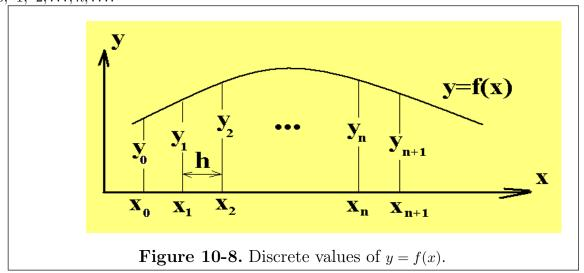
Define the second forward difference as a difference of the first forward difference. A second difference is denoted by the notation  $\Delta^2 y_n$  and
