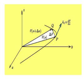
Let s denote the distance along a curve measured from some fixed point on the curve and let the position vector of a point P on the curve be represented as a function of this distance. If the position vector is given by
