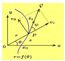
Consider the motion of a particle which is described in polar coordinates by an equation of the form  $r = f(\theta)$ , where  $\theta$  is measured in radians. Select a point P with coordinates  $(r, \theta)$  on the curve and construct the radius vector  $\vec{r}$  from the origin to the point P. Construct the tangent to the curve at the point P and define the angle  $\psi$  between the radius vector and the tangent. Label a fixed point on the curve, say
