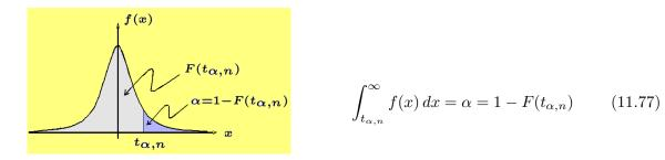
The normal distribution is related to the student's t-distribution as follows. If  $\overline{x}$  and s are the mean and standard deviation associated with a random sample of size n from a normal distribution  $N(x; \mu, \sigma^2)$ , then the quantity  $\frac{(\overline{x} - \mu)\sqrt{n}}{s}$  has a student-t-distribution with n-1 degrees of freedom.
