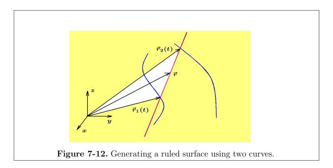
For a fixed value of the parameter t, one can draw a straight line between the two points  $\vec{r}_1(t)$  and  $\vec{r}_2(t)$  as illustrated in the figure 7-12. If  $\vec{r}$  is the position vector to a general point on this line it can be represented by the equations
