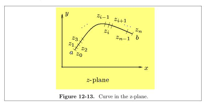
The curve C is assumed to be a smooth curve represented by a set of parametric equations
