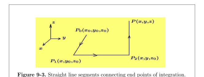
Along the sectionally continuous straight-line paths of integration illustrated in figure 9-3 the line integral (9.45) can be expressed in the component form as
