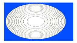
An example of a two-dimensional scalar field is a scalar function  $\phi = \phi(x, y)$  representing the temperature at each point (x, y) inside some specified region. The scalar field can be visualized by plotting the family of curves  $\phi(x, y) = C$  for various values of the constant C.
