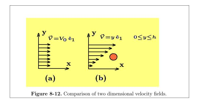
In comparison, consider the two-dimensional velocity field  $\vec{V} = y \hat{\mathbf{e}}_1$ ,  $0 \le y \le h$ , which is illustrated in figure 8-12(b). Here the velocity field may be thought of as representing the flow of fluid in a river. The curl of this velocity field is
