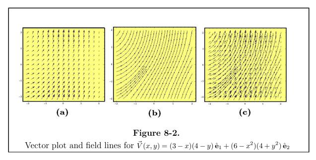
The figure 8-2 illustrates three graphs created by a computer. The figure 8-2(a) represents a vector field plot over the region  $-2 \le x \le 2$  and  $-2 \le y \le 2$ . The figure 8-2(b) is a graph of the field lines associated with the vector field with arrows placed on the field lines. The figure 8-2(c) is the vectors of figure 8-2(a) placed on top of the field lines of figure 8-2(b) to compare the different representations.
