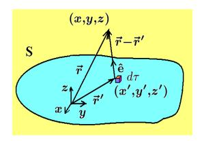
Consider a volume V enclosed by a surface S as illustrated and let  $\vec{J} = \vec{J}(x', y', z')$  denote the current density within this volume. Let (x', y', z') denote a point inside V where an element of volume dV = dx'dy'dz' is constructed. In addition, construct the vectors  $\vec{r} = x \, \hat{\mathbf{e}}_1 + y \, \hat{\mathbf{e}}_2 + z \, \hat{\mathbf{e}}_3$  to a general point (x, y, z) outside of the volume V and
