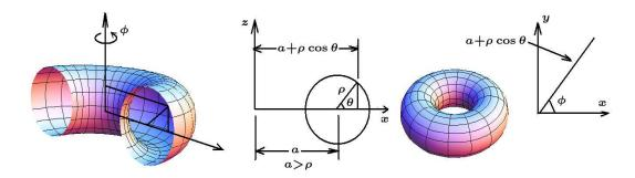
$dS = \rho(a + \rho\cos\theta)\,d\theta\,d\phi$  and  $dV = \rho(a + \rho\cos\theta)\,d\rho\,d\theta\,d\phi$  Volume is  $V = 2\pi^2a\rho^2$  and surface area is  $S = 4\pi^2a\rho$
