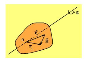
Let  $\vec{B}$  denote any vector connecting two fixed points within a rigid body which is rotating about a line with angular velocity  $\vec{\omega}$ . Let  $\vec{r}_1$  denote a vector to the terminus of  $\vec{B}$  and let  $\vec{r}_2$  denote a vector to the origin of  $\vec{B}$ , as measured from some origin on the axis of rotation. One can then write
