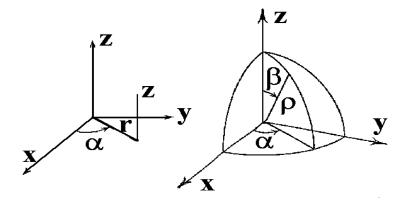
Figure 1.1-5. Cylindrical and Spherical Coordinates
